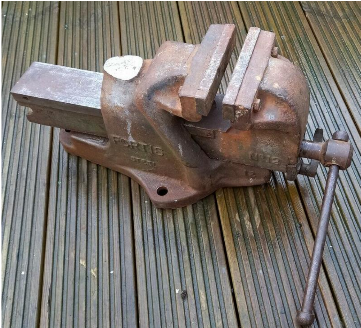
Ebay 2022 Steel No12 later shaped design casting but no "Unbreakable". Egg shaped anvil flat hub for bar
