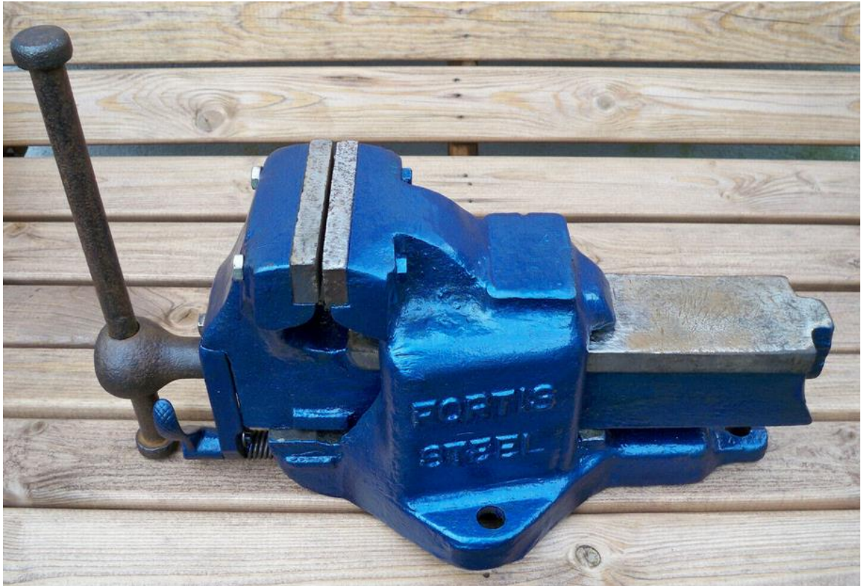
Ebay 2022. No10 "The" is dropped – Fortis Steel. Side plates added. Round hub for bar.
