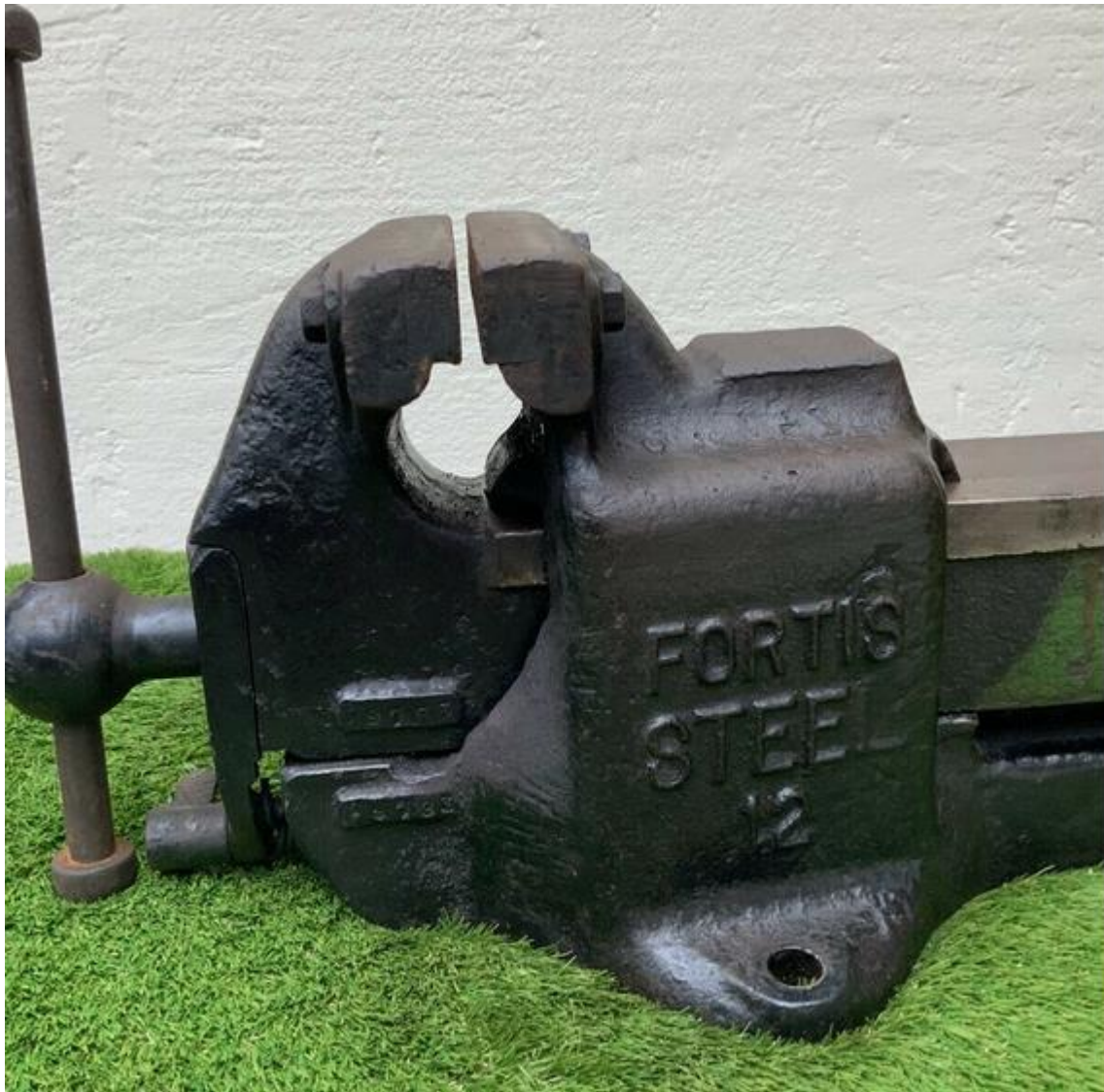
Ebay 2022. No 12. VM cast into base and extra 12 cast (now in 3 places) Round hub. Production numbers punched onto side plates. Rectangular anvil.
