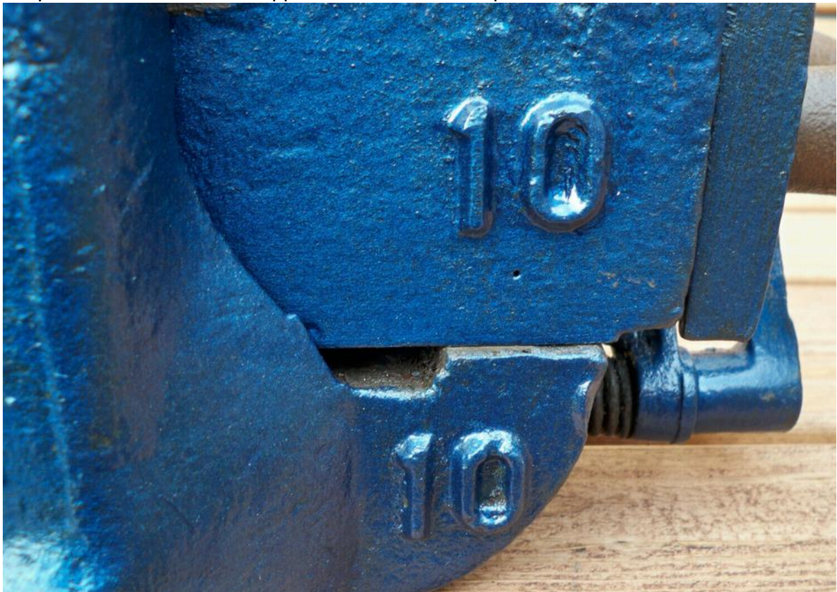
Ebay 2022. No10 "The" is dropped – Fortis Steel. Side plates added. Round hub for bar.
