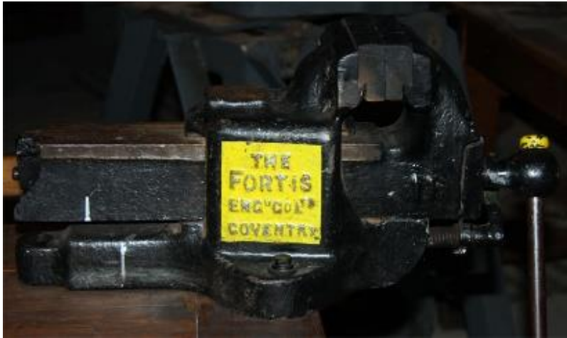
(Fortis Engineering, n.d.) Seems 1st or 2 nd generation with plate affixed to side. Round hub for bar.
