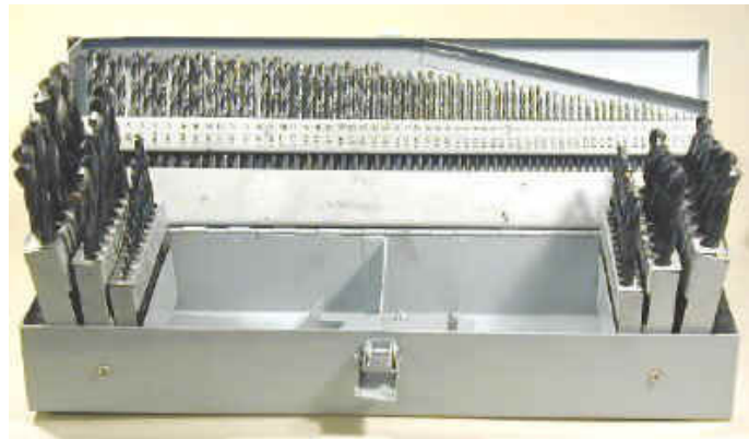
Set of 119 fractional, number and letter drills.
