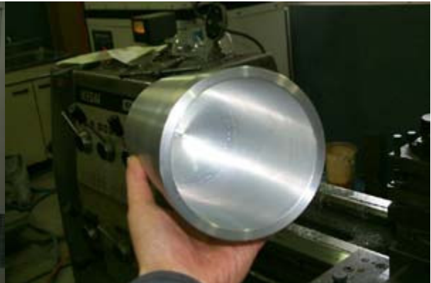
(6) The boring processing is finished. It has a beautiful surface finish.
