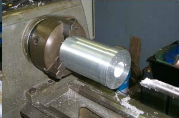
(2) The hole is spread with a boring bar.
