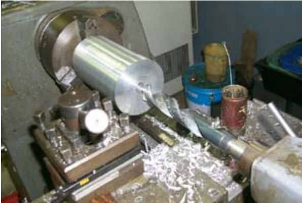
(1) An undersized hole is made with a drill.
