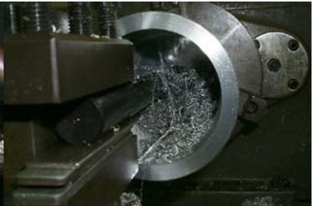
(4) It is hard to see the inner surface because of swarf.
