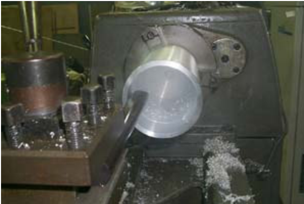
(5) As the diameter is enlarged, cutting of the thin material becomes harder.
