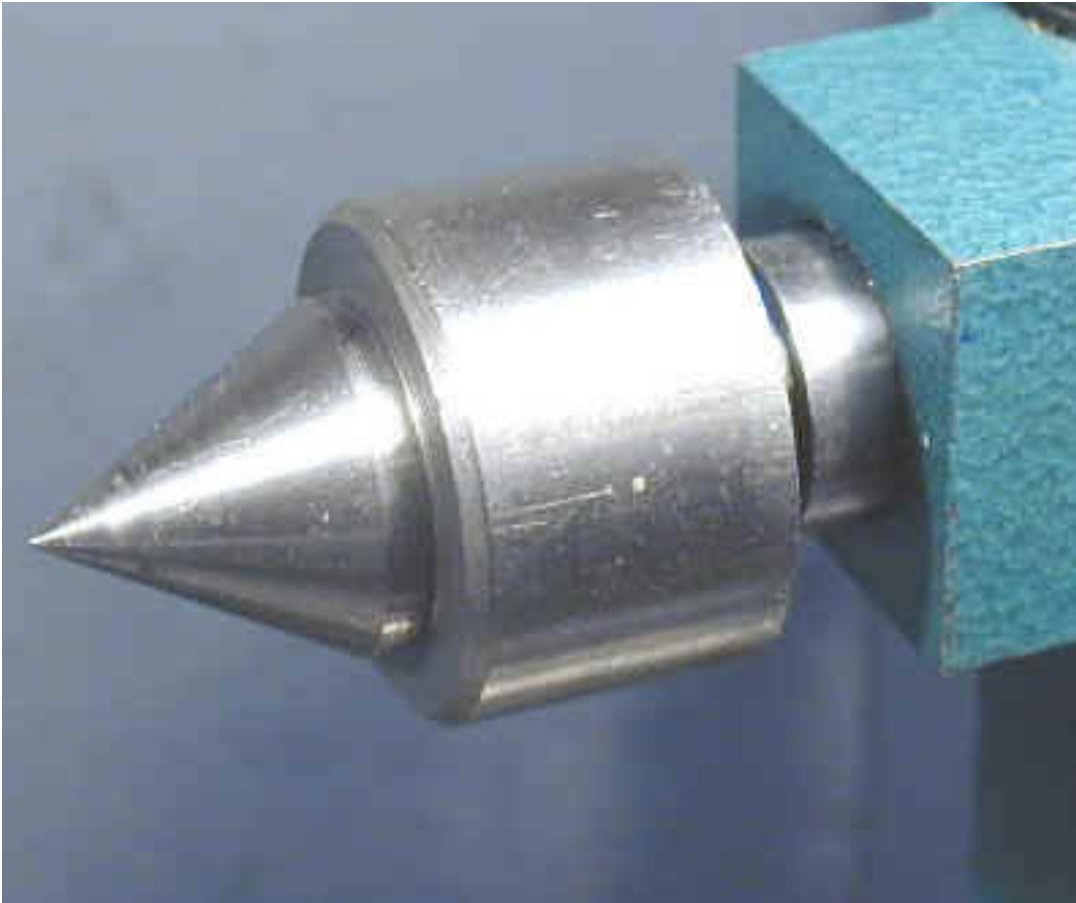
Live Center mounted in tailstock ram
