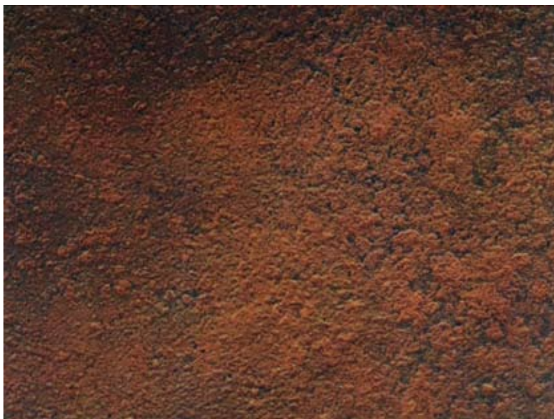
Preparation Grades. Scraping and wire-brushing D St 2
