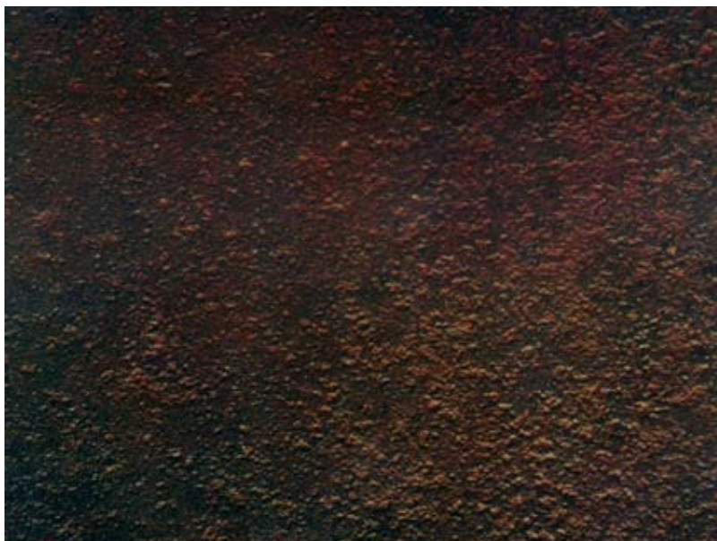
Preparation Grades. Scraping and wire-brushing D St 3
